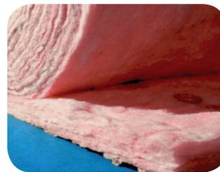
on the attic floor before pouring or blowing in loose-fill insulation. Or you can purchase batt insulation with a kraft paper or foil vapor barrier attached. Be sure to install this type of vapor barrier closest to your living space.
