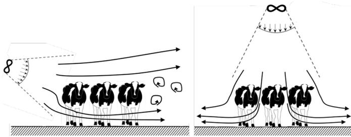
**Figure 4.** Temperature (left) and air velocity (right) resulting from panel fans cooling cows.
