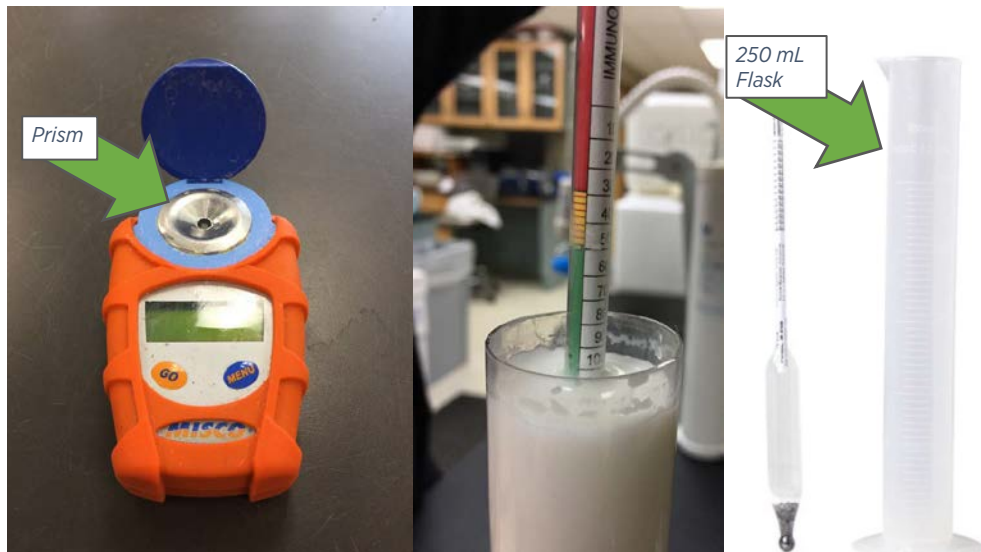
Photo 2. Left: A digital refractometer. A few drops of colostrum are placed on the prism and the percent sugar in aqueous solutions is provided to determine colostrum quality. Middle: A hydrometer colostrometer measuring colostrum quality using color. In the pictured example, this colostrum is green quality (greater than 50 mg/mL of Ig). Right: Be sure to use an appropriate 250 mL flask to measure colostrum quality.
