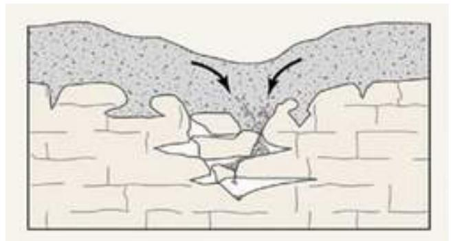
Figure 4: Soil subsidence in the absence of tree roots
