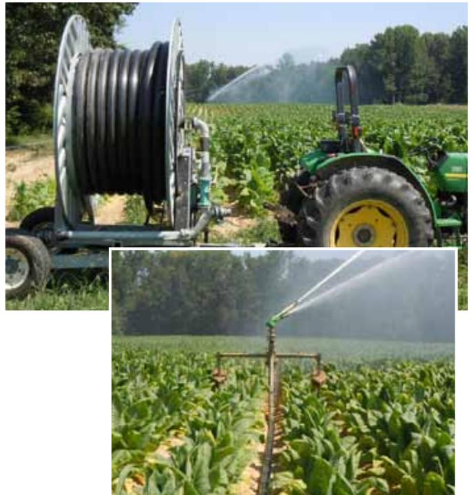
*Traveling gun irrigation in tobacco with close-up of sprinkler and cart*
