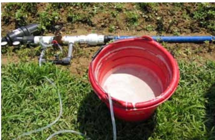
*Check Valve, Injector, Screen Filter, and Batch Tank for Fertigation*
