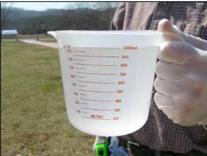
Figure 22. Measuring the amount of water collected from one tip for the amount of time in seconds required to complete the calibration course.
