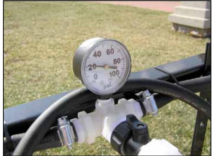
*Figure 4. The main pressure gauge is most often located where it is easily viewed by the operator.*
