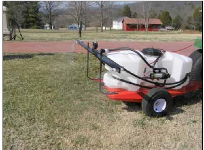
Figure 18. Determining the total width of the boom spray pattern.
