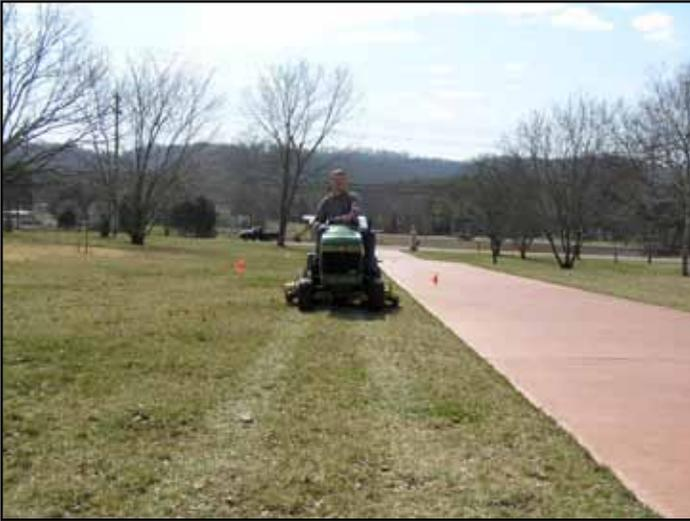
Figure 20. Recording the amount of time required for the tractor and attached sprayer to move through the calibration area.
