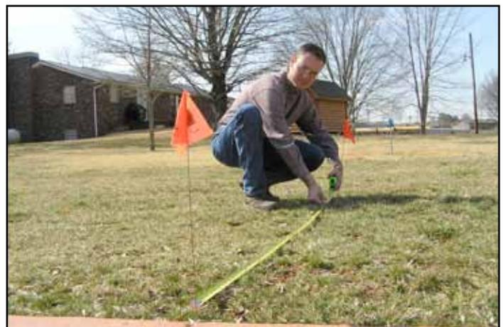
Figure 19. Measuring and marking the calibration course.
