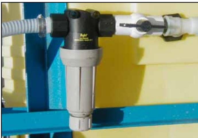
*Figure 3. In-line strainers capture particulate matter that may clog tips or restrict solution flow and are plumbed between tank and positive-displacement pumps.*
