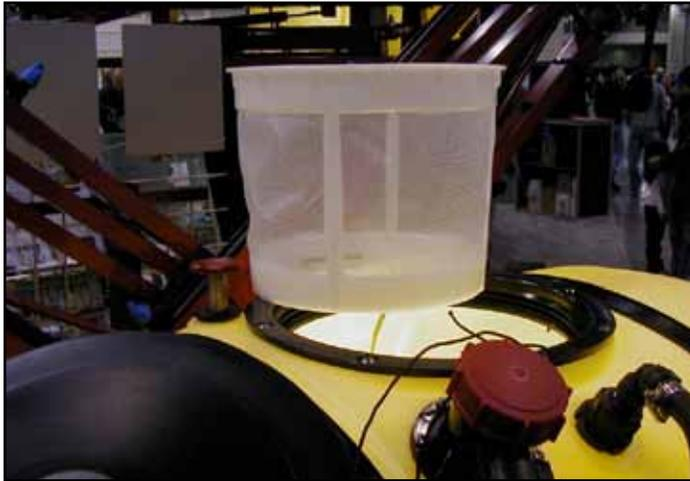
*Figure 2. Basket-type screens prevent debris from entering sprayer tank during fill-up.*
