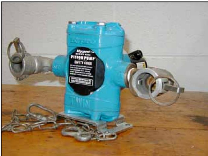
Figure 7. Another type of positive-displacement pump is a piston pump, which has low flow and medium-to-high pressure capacities.
