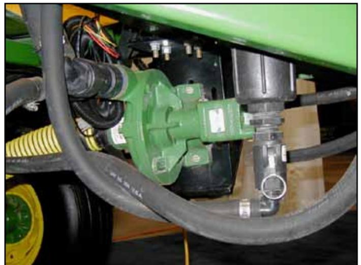
Figure 9. A centrifugal pump is classified as a non-positive displacement pump with medium-to-high flow and low-to-medium pressure capacities.
