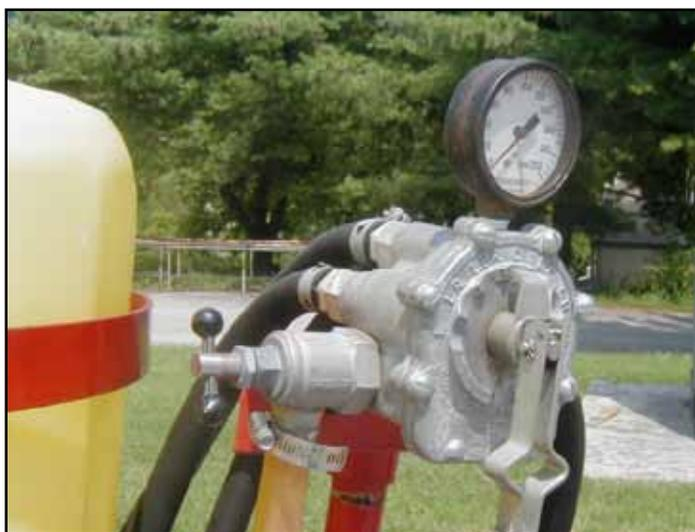
Figure 15. A pressure relief/regulating valve is a required component for sprayers equipped with positive displacement pumps.
