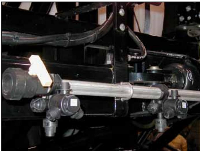
Figure 12. A wet boom is hollow and carries solution directly to spray tips.
