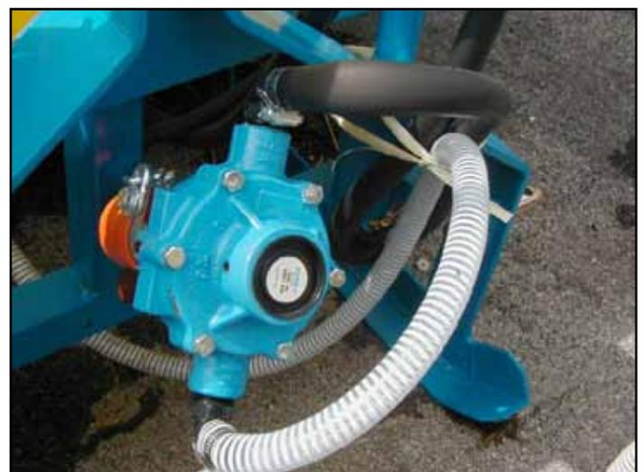
Figure 13. Both suction- and pressure-type hoses are used on sprayers to deliver solution from the tank to the spray tips.
