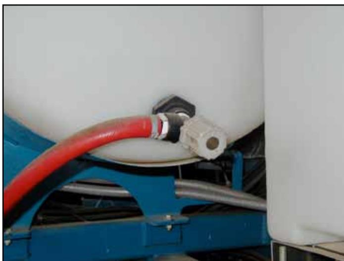
Figure 16. A manual throttling valve is usually located between the pump and jet agitator, mounted inside the tank, providing independent control of the amount of hydraulic agitation.
