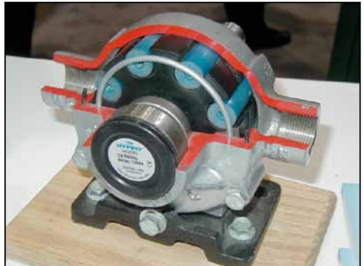
Figure 8. A roller pump is classified as a semi-positive displacement pump and is considered to have medium flow and pressure capacities.
