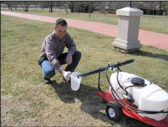
Figure 21. Collecting the amount of water from one tip for the amount of time in seconds required to complete the calibration course.
