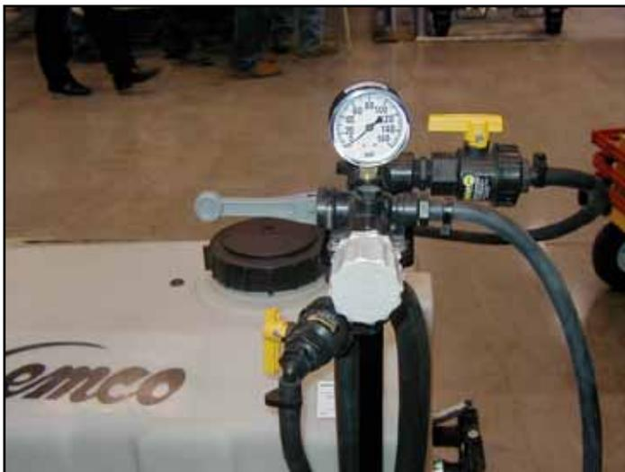
Figure 14. A variety of valve types are used on sprayers to control system pressure, flow direction and flow rates.
