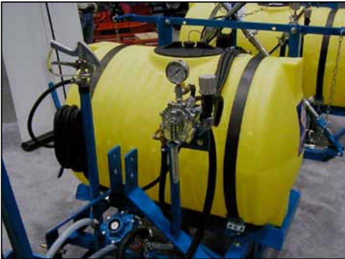
Figure 5. The spray tank is usually mounted above the pump to improve priming.
