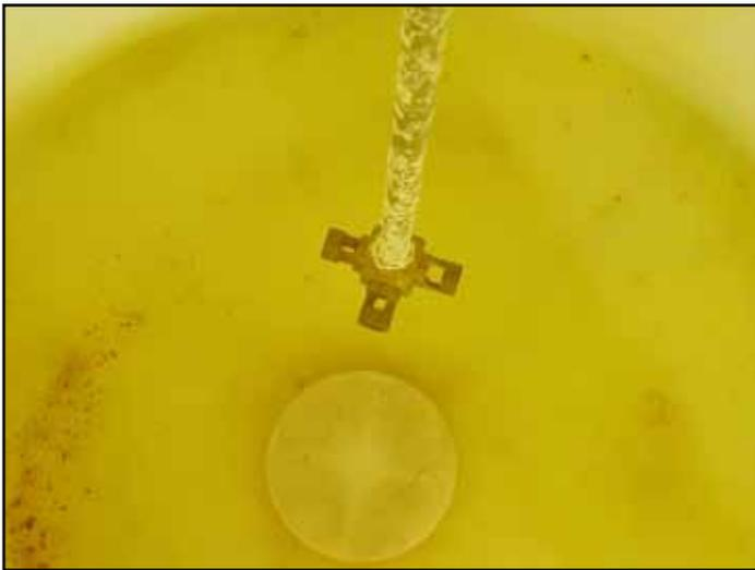
Figure 10. Hydraulic agitators stir solutions by re-circulating flow back to the tank.
