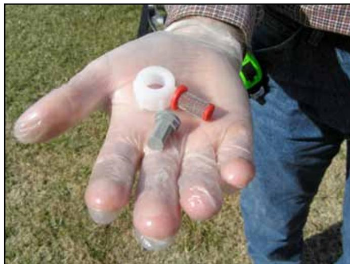
*Figure 1. Spray nozzle tip and strainer are held in place by a nozzle body cap.*
