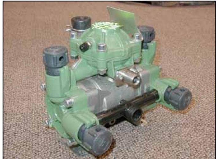
Figure 6. A diaphragm pump is classified as a positive-displacement pump with low-to-medium flow and medium-to-high pressure capacities.
