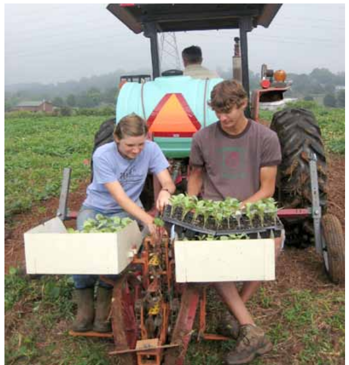
The no-till transplanter sets plants without cultivating the soil.
