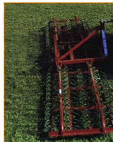
spacing vary among machines. The blades or tines dislodge and lift thatch as the vertical mower or 'dethatcher' moves across the turf. Vertical mowers are adjusted such that the blades or tines penetrate the thatch layer and lightly contact the soil below. After dethatching, a vacuum or blower may be used to
