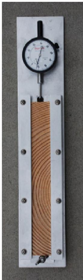
involved measuring the swelling of wood samples after 30 minutes of submersion in water. The coated samples were then compared to the bare-wood controls. Each water-repellent product was tested on ten samples of southern pine wood.
