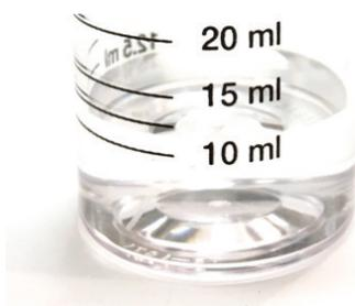
End-point of the PAA titration, a colorless solution. The number of drops of titrant added indicates the concentration of PAA.
