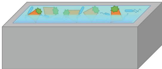
During washing, some foodborne pathogens will fall off the contaminated produce and into the wash water where they can cross-contaminate other produce they contact.
