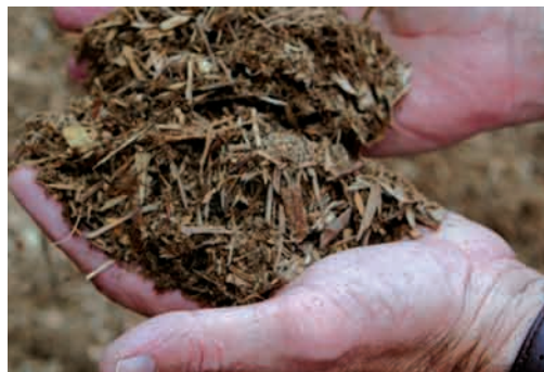
Woody residues such as this hog fuel are the largest source of renewable energy used in the United States.
