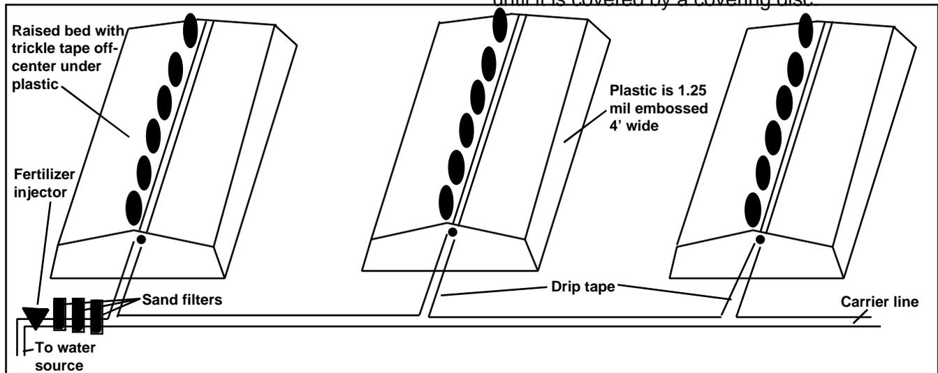
Figure 1. Illustration of trickle irrigation and plastic system.
