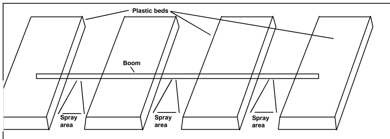
**Figure 4. Illustration of a directed spray for weed control when cantaloupes are being produced on plastic.**
