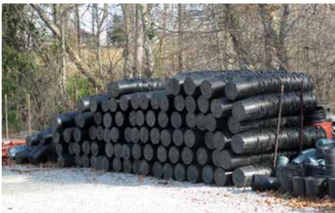
**Figure 2. Good Example: Containers are stored on gravel, preventing contact with soil or puddled water.**
