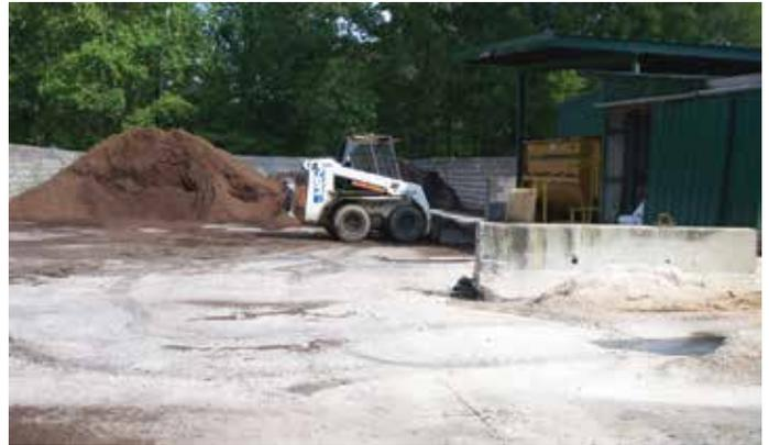
**Figure 4. Good Example: Substrate is stored on a well-drained container pad with dedicated equipment to prevent contamination from soil.**
