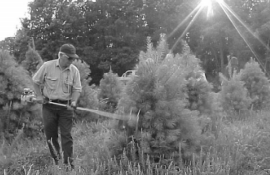
Small gasoline-powered shearing machine.
