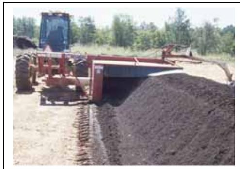
**Figure 6. Turning a windrow- with a tractor mounted windrow turner**
