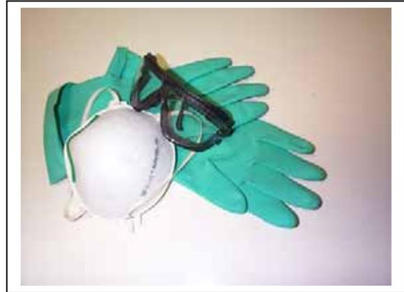
**Figure 4: Workers should use protective wear: goggles, gloves and dust masks, when handling and applying alum**
