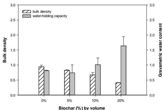
Figure 3. Bulk density and water-holding capacity (gravimetric water content at field capacity) of biochar-amended soils based on biochar concentration (Ashworth, 2014; unpublished data).
