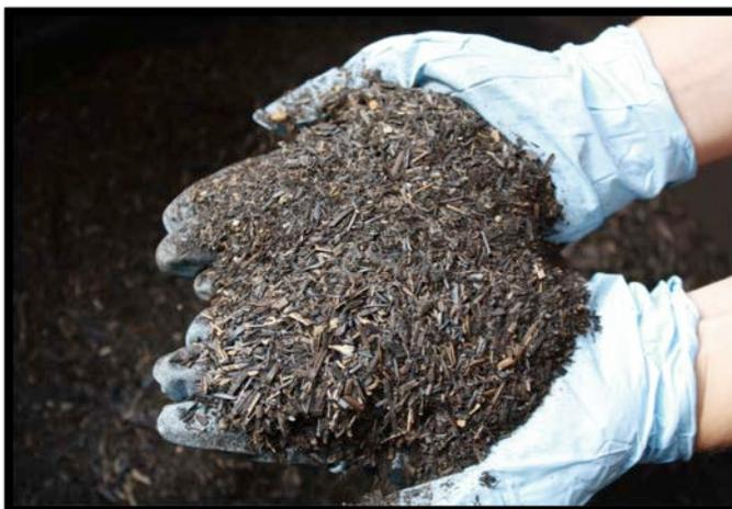
Figure 1. Biochar produced from switchgrass via pyrolysis at 400 C.
