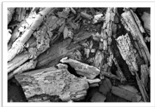
Figure 2. Scanning electron micrograph of switchgrass-biochar.
