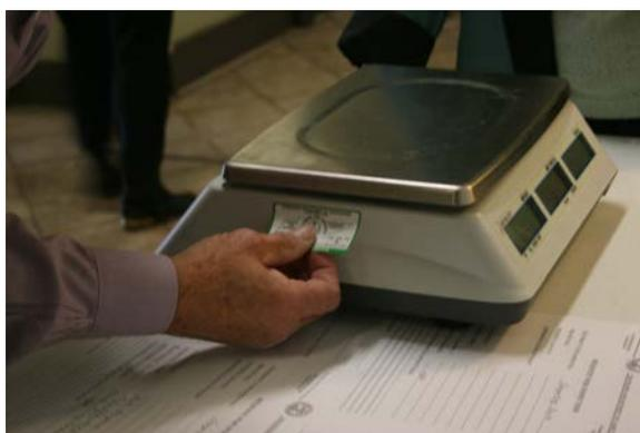
Figure 2. If the scale passes inspection, the TDA WM inspector applies a certification sticker to the scale, verifying that the scale has been officially examined and approved by the TDA.
