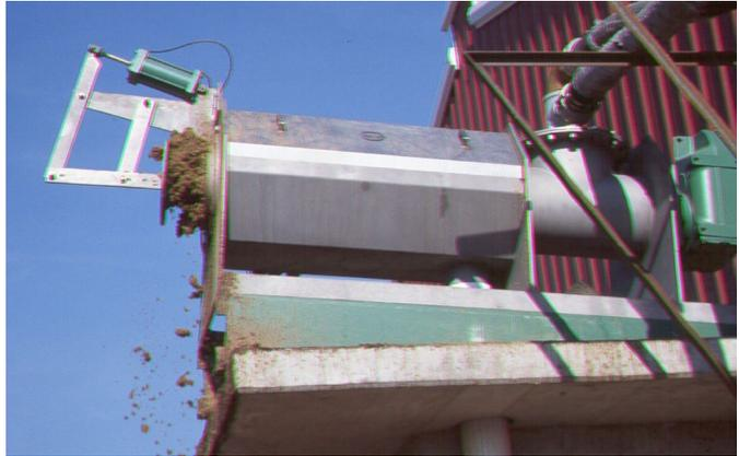
Figure 4. Screw-press separator. Source: Author Photo
