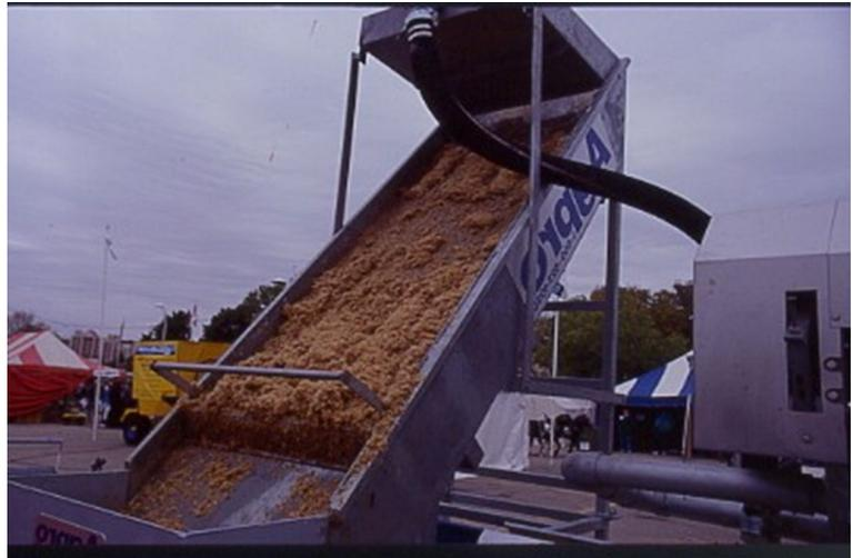
Figure 2. Static-screen separator. Source: Author Photo
