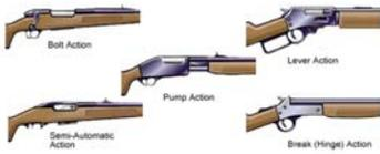
This slide illustrates the different types of actions normally seen in long guns. The action actually contains the fire control mechanism and controls the cartridge while it is being fired. When we say 'keep the action open' this is the part of the firearm we are talking about.
